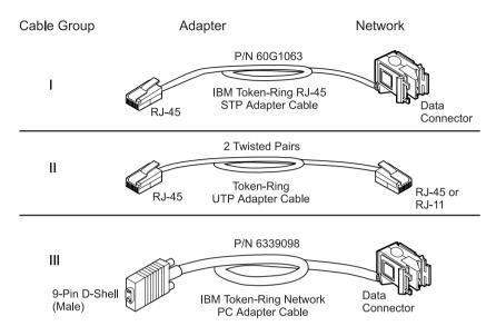
Figure 2-3. STP and UTP Adapter Cables
