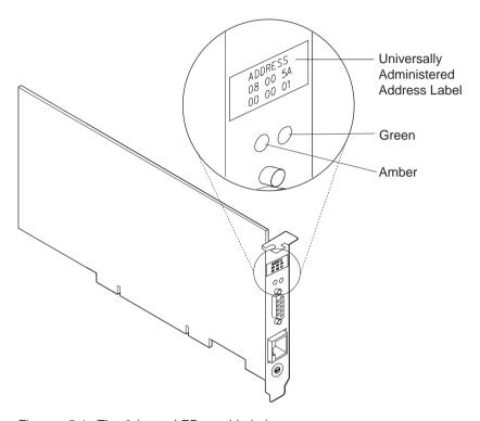
Figure 5-1. The Adapter LEDs and Labels
