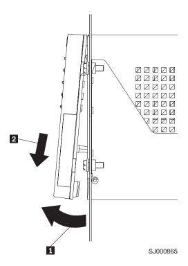
Figure 9. Removing the controller-unit bezel (machine types 3552 and 1742)
