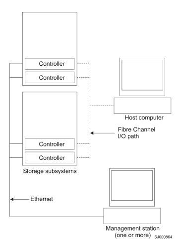
Figure 3. Direct-management (out-of-band) storage subsystems
