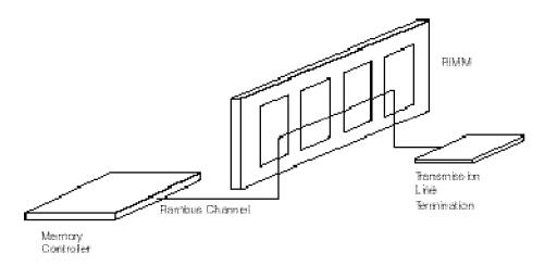
Data transfers are organized into packets of 16 bytes. Consequently eight data transfers occur for each packet over a period of four clock cycles. (This takes 10 nanoseconds at the 800Mbps bit rate.) Internally the RDRAM chip is organized as a 128-bit wide data flow, allowing the entire 16-byte transfer to be generated from a single access.
