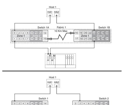
Figure 37. Switch zoning in cascaded (top) and noncascaded (bottom) fibre-channel switches
