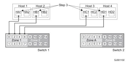
Figure 50. Connecting the primary host bus adapter (Hx1) to the fibre-channel switches
