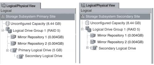
Figure 29. Mirrored logical drive pair showing Unsynchronized status
