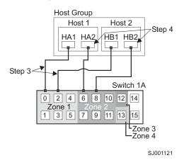
Figure 45. Connecting the host bus adapter to fibre-channel switches
