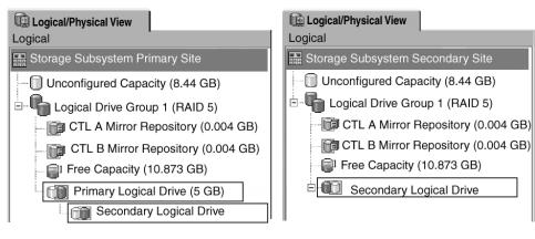
Both the primary and secondary logical drives are displayed in the Subsystem Management window for the storage subsystem. Only the secondary logical drive is displayed in the Subsystem Management window for the secondary storage subsystem.
