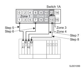
Figure 46. Connecting the storage subsystem to fibre-channel switches
