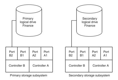
Figure 33. Controller B shown as controller owner
