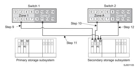
Figure 53. Connecting the secondary storage subsystem to fibre-channel switches
