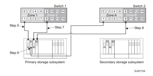
Figure 52. Connecting the primary storage subsystem to fibre-channel switches
