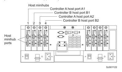
Figure 31. Controller A and Controller B host ports
