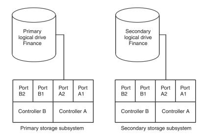
Figure 32. Controller A shown as the controller owner
