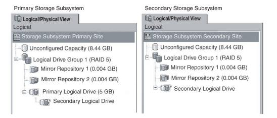
Figure 30. Mirrored logical drive pair showing Synchronization-in-Progress status
