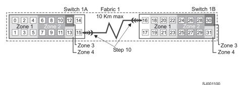
Figure 47. Connecting fibre-channel switches over a remote network to complete the Fabric 1 environment
