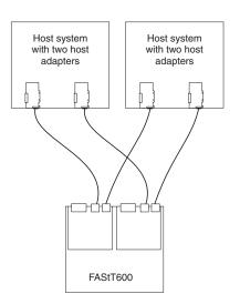
Figure 19. Redundant host and drive Fibre Channel loop configurations
