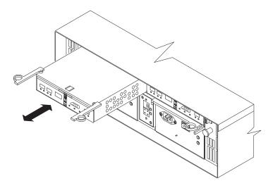
Figure 49. Pull-rings for removing a controller
