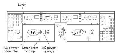
Figure 56. Lever for power supply removal
