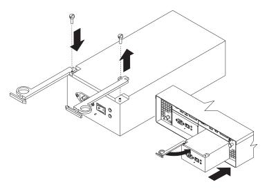
Figure 57. Installing a hot-swap power supply
