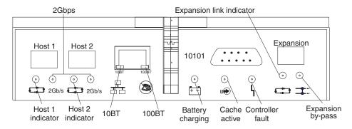
Figure 36. RAID controller LEDs
