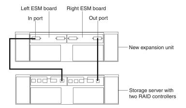
Figure 33. Adding an expansion unit
