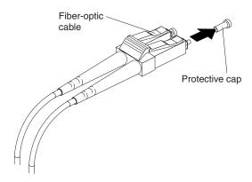
Figure 27. Removing caps from fiber-optic cables
