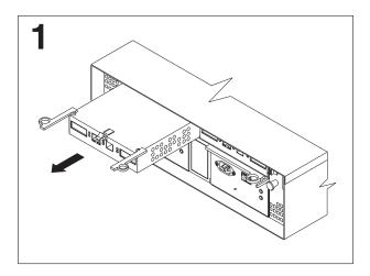
Figure 8. RAID controller removal
