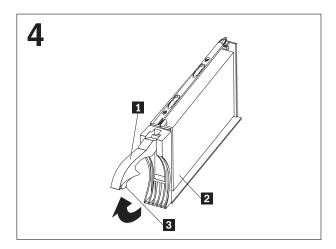
Figure 11. Hard disk drive removal
