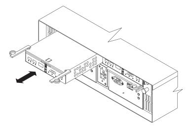
Figure 63. Pull-rings for removing a controller
