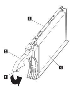
Figure 51. Releasing the drive latch
