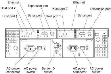
Figure 4. Interface ports and switches
