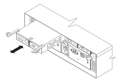
Figure 66. Installing a new RAID controller
