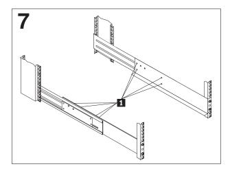
Figure 14. Rail adjustment screws
