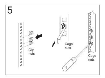
Figure 12. Rack nut installation
