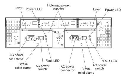
Figure 55. Power supply controls
