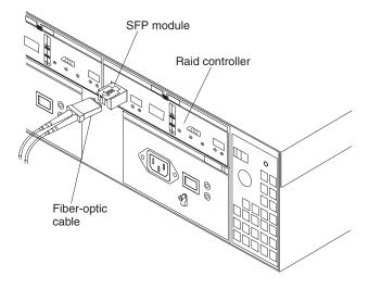
Figure 46. Location of SFPs and fiber-optic cables
