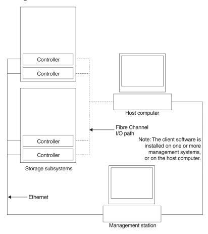
Figure 18. Direct-managed storage subsystems
