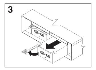
Figure 10. Power supply removal
