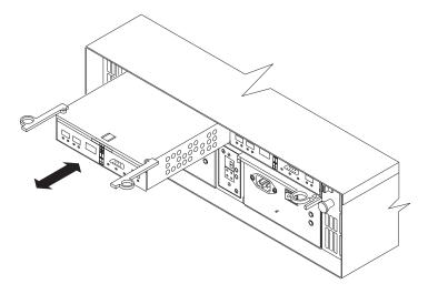
Figure 44. Pull-rings for removing a controller
