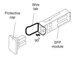
Figure 48. Unlocking the SFP module latch - wire variety
