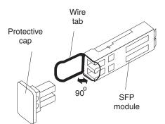
Figure 43. Unlocking the SFP module latch - wire variety
