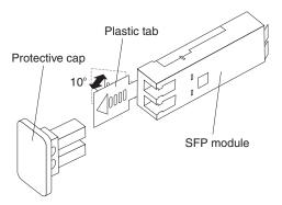
Figure 61. Unlocking the SFP module latch - plastic variety
