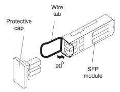
Figure 62. Unlocking the SFP module latch - wire variety
