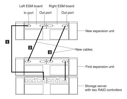
Figure 34. Adding a second expansion unit
