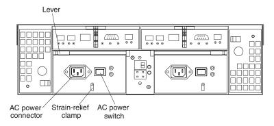
Figure 58. Connecting the power cord to the AC power connector
