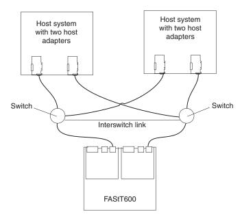
Figure 20. Single SAN fabric zone configuration
