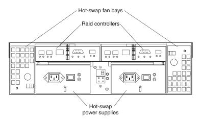
Figure 3. Back view of FAStT600 storage server
