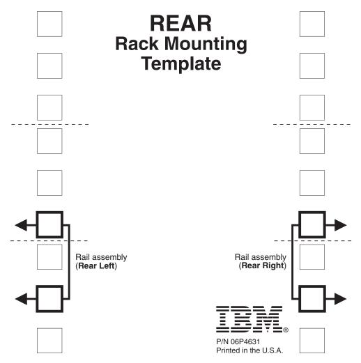
Figure 7. Rear rack mounting template
