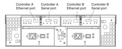
Figure 30. Ethernet and serial port locations
