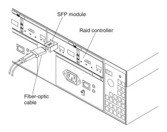
Figure 60. Location of SFPs and fiber-optic cables
