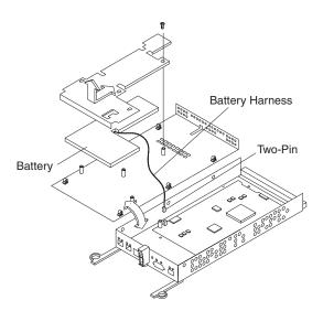
Figure 65. Removing the controller battery
