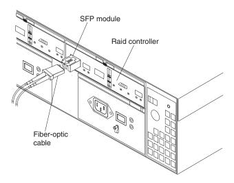
Figure 41. Location of SFPs and fiber-optic cables
