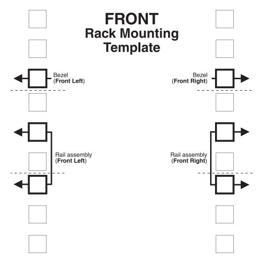
Figure 6. Front rack mounting template
