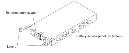
Figure 40. RAID controller levers and labels
