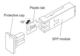
Figure 47. Unlocking the SFP module latch - plastic variety
