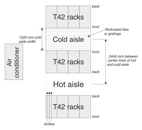
Figure 5. Example of Cold Aisle/Hot Aisle rack configuration
