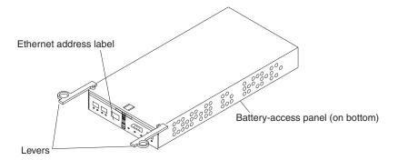
Figure 45. RAID controller levers and labels
