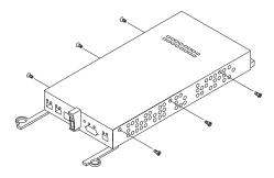
Figure 64. Controller battery-access panel screws
