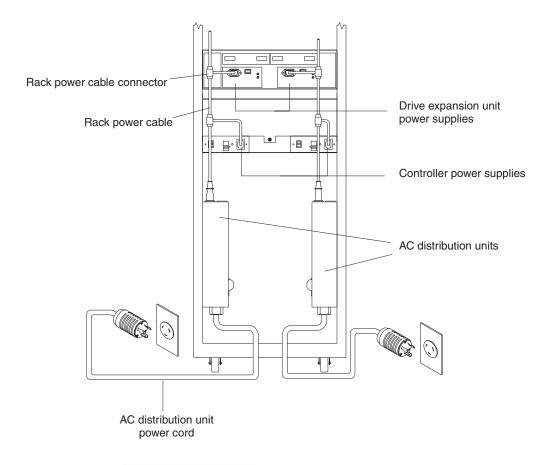
Figure 32. Redundant AC power connections to controllers and drive expansion units
