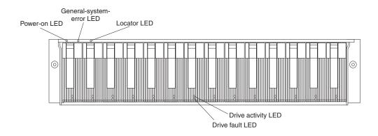
Figure 35. Storage server LEDs (front)
