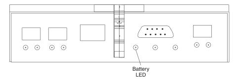
Figure 39. Battery LED
