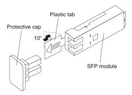
Figure 42. Unlocking the SFP module latch - plastic variety
