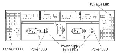
Figure 37. Fan and power supply LEDs
