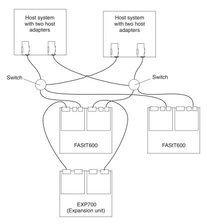
Figure 21. Dual SAN fabric zone configuration
