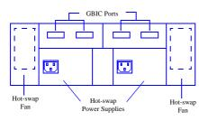
• Two hot-swap, 350 W auto-ranging, redundant power supplies. Redundant fans - two hot-swap, dual-fan units.
