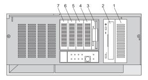
The server comes with a CD-ROM drive installed in bay 2 and a diskette drive installed in bay 3. Some models come with a preinstalled hard disk drive.
