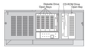
**Open Bays:** Your server's design accommodates 3.5-inch and 5.25-inch devices, such as hard disk, tape, and rewritable optical disk drives. The number and capacities of the hard disk drives vary by model.
