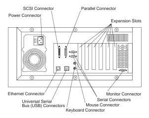
PC Server 326 Type 8639 Models 1RY, 2RY, PB0, and RBO come with auto-sensing power supplies. There is no voltage select switch on the power supply.
