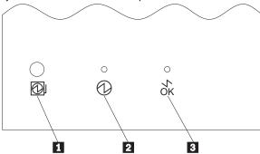
The Power Status LED 2 On indicates power is enabled to the system. The Power Status LED Off indicates power is disabled to the system.
