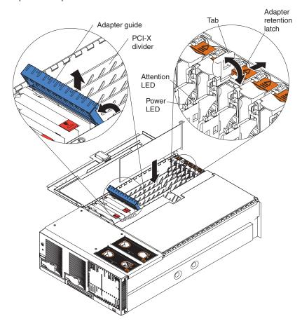
4. Follow the cabling instructions, if any, that come with the adapter. Route the adapter cables before you install the adapter.
