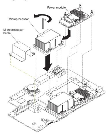
c. Ensure that the socket lock is in the fully open (unlocked) position to permit plugging in the microprocessor. Use the hex wrench provided with the microprocessor option to open the lock, if necessary.
