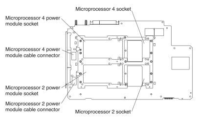
**Important:** To ensure proper server operation after you install replacement or additional microprocessors, install only microprocessors that have the same cache size and type, and the same clock speed. For a list of microprocessors supported by your server, go to the ServerProven list at <a href="http://www.ibm.com/pc/us/compat/">http://www.ibm.com/pc/us/compat/</a>.
