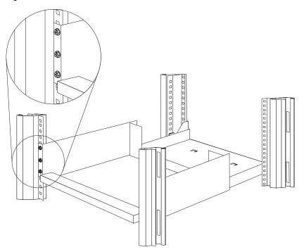
The monitor compartment installation is complete. You can now install your monitor in the compartment.
