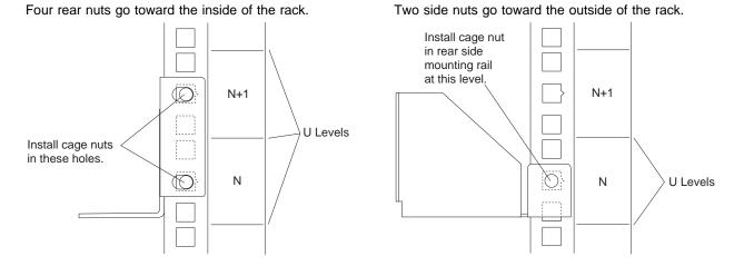
1) Hook one side of the cage-nut clip into the rack-mounting-rail square hole.
