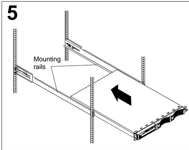
Place the computer on the mounting brackets and slide it into the rack as far as it will go.
