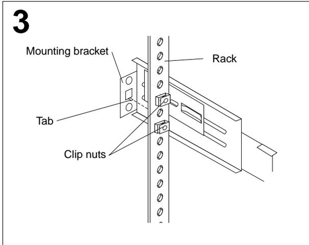
Insert the bracket tab through the center hole between the two clip nuts on the rear rail. (The right and left rails are labeled.)
