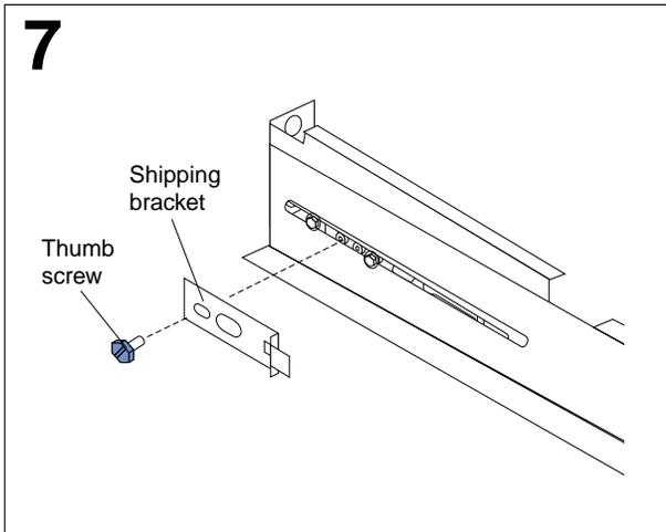
If you want to ship your rack with the computer installed, you must install the shipping brackets on each side of the computer. This is done by inserting the shipping bracket tab into the slot on the back of the computer. Then, use the blue thumb screw to secure the back of the computer and the shipping bracket to the mounting bracket.
