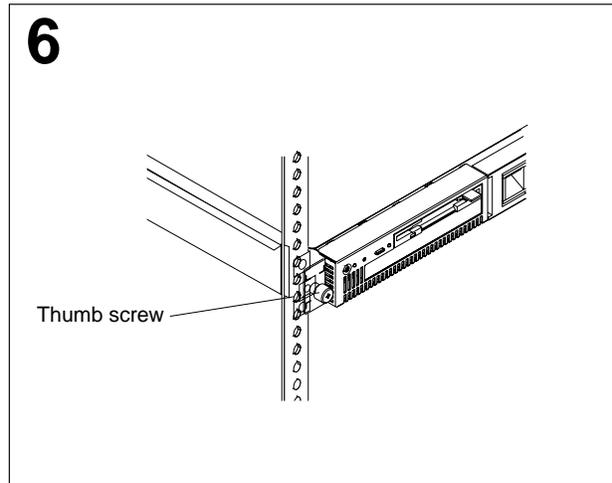
Tighten the thumb screws on the front of the computer to secure it to the rack.
