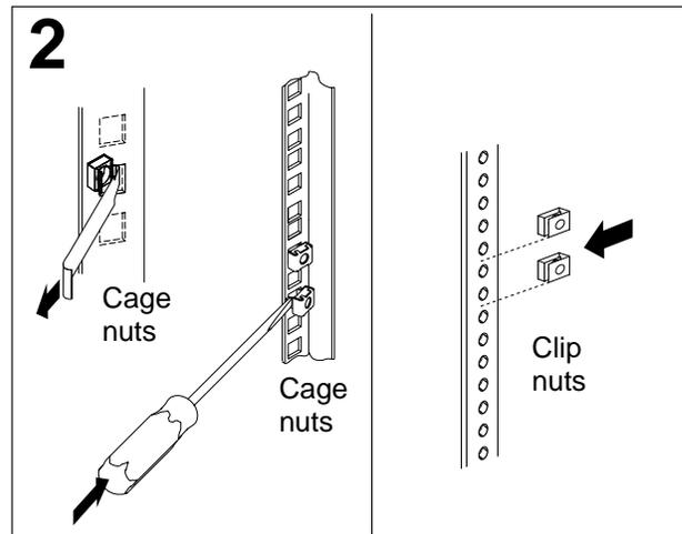
Select a 1 U size location in the rack. Install a cage nut or clip nut in the top and bottom position of the 1 U location you selected (both sides, front and rear of the rack).
