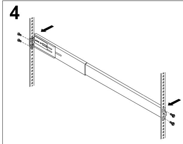
Loosely install two mounting screws through the back end of the bracket. Position the mounting bracket so that it lines up with the clip nuts. Install the remaining mounting screws, then tighten all the screws with a screwdriver. Repeat these steps for each mounting bracket.
