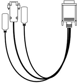
You can manage your server remotely from another computer on the network or locally with a keyboard, monitor, and mouse or other pointing device connected to your server. If you manage your server locally, you must use the C2T device breakout cable. Connect the large connector on the C2T cable to the rear of your server; then, connect your keyboard, mouse, and monitor to the connectors on the other end of the C2T cable.
