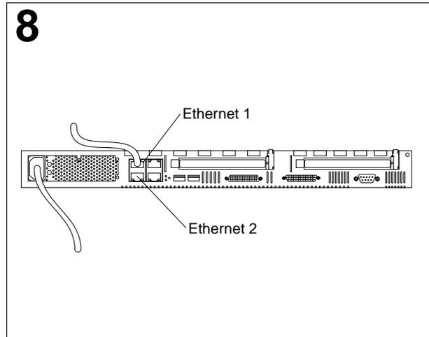
Connect the power cord; then, connect Ethernet cables to the management adapter as follows:
