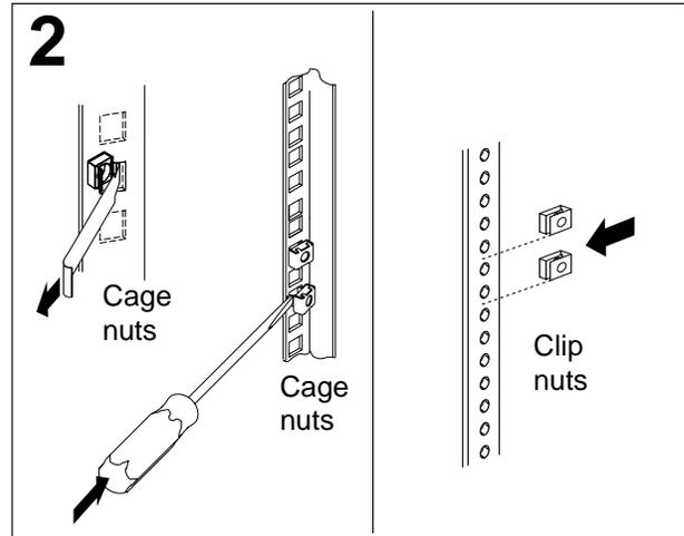
Select a 1 U size location in the rack. Install a cage nut or clip nut in the top and bottom position of the 1 U location that you selected (both sides, front and rear of the rack).
