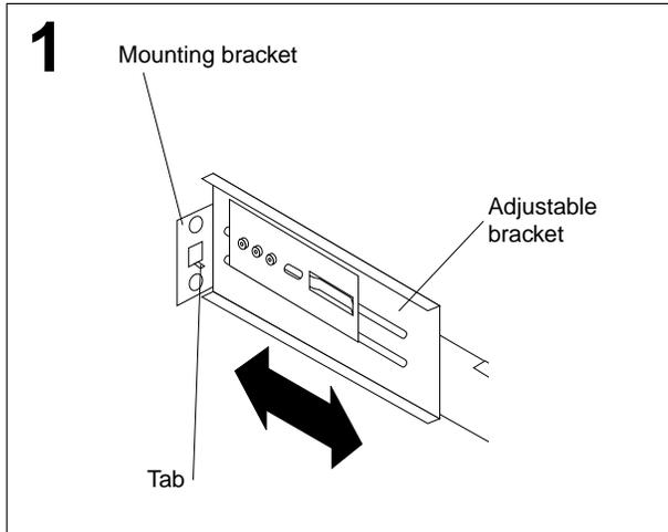
Adjust each rear mounting bracket (by loosening the screws) so that the inside distance between the two ends is equal to the outside dimension of the rack rails.
