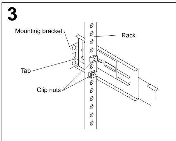
Insert the bracket tab through the center hole between the two clip nuts on the rear rail. (The right and left rails are labeled.)
