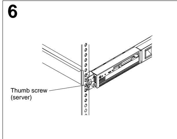
Tighten the thumb screws on the front of the server to secure it to the rack.
