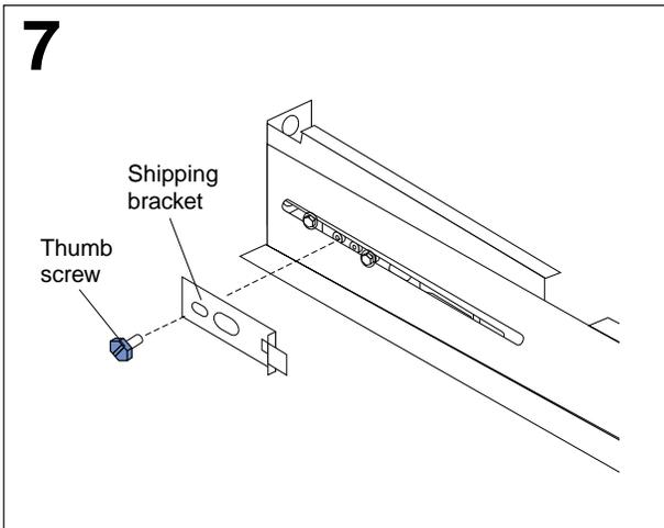
If you want to ship your rack with the server installed, you must install the shipping brackets on each side of the server. To do this, insert the shipping bracket tab into the slot on the back of the server. Then, use the blue thumb screw to secure the back of the server and the shipping bracket to the mounting bracket.
