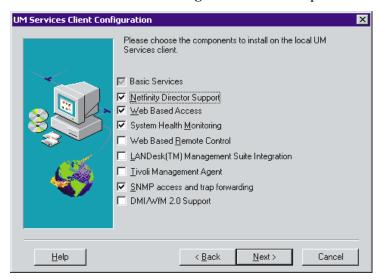
2. Check the checkbox beside any of the components you want to install on the client system. All of the components, except for Netfinity Director Support, are described under "Installing the Server Files" on page 10. For an explanation of these components see pages 11-13.
