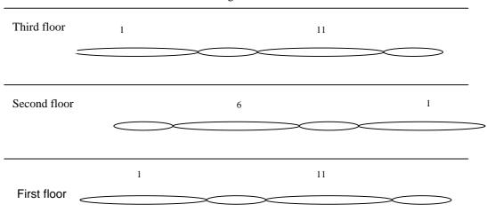
In this way access points with the same frequency cannot hear each other, so they don't take each others bandwidth. In multi-story buildings, you can also identify the vertical point-to-point distance, to determine the range of access points across multiple floors.
