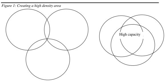
Increasing the overlap of wireless cells as pictured in the right side of Figure 1, enables you to create a high capacity network, where numerous mobile wireless stations can engage in heavy traffic loads, or roam at velocities higher than pedestrian speed. If each of the wireless cells is assigned a distinct operating frequency, this type of network enables you to triple the average throughput capacity in a specific environment.
