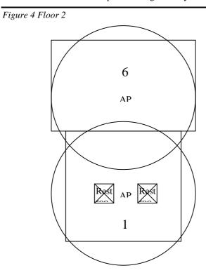
On floor 2 are two APs with frequencies offset from floor 1. When all circles are drawn, this will indicate the number of access points that must be procured.
