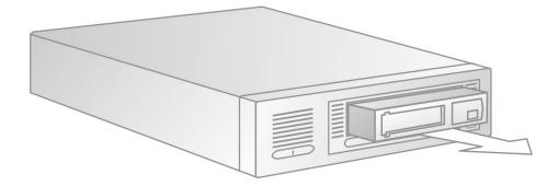
3. After the tape cartridge ejects, grasp the cartridge and remove it.
