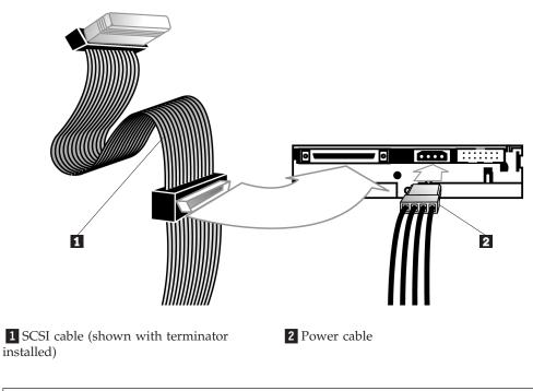
**Note:** The SCSI adapter might be part of the computer system board or might be an adapter installed in an expansion slot.
