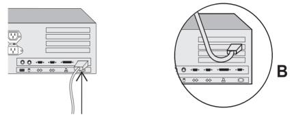
3. Connect the power cord to the power port on the back of your monitor if the power cord supplied is not attached to the monitor. Then insert the plug into a properly grounded electrical outlet.
