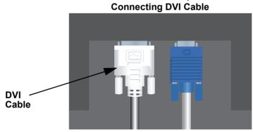
5. Connect the DVI connector at the other end of the signal cable to the DVI port located on the back of the graphics adapter. See picture below.
