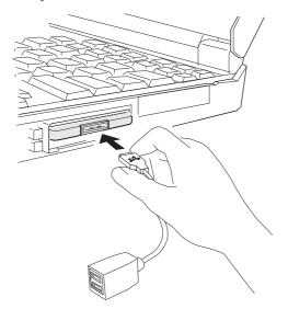
**Attention:** The adapter cable has pins for proper alignment into the ThinkPad USB 2.0 CardBus Adapter connector and should gently click into place. Do not force the connection. Forcing the connection might cause damage to either the card or the cable end.
