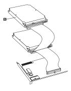
The connector on one end and the connector in the middle connect to the storage devices. The other end of the cable connects to the IDE port. The IDE port can be on the computer system board or on an adapter installed in an expansion slot. For the best signal quality when you have only one device on the IDE cable, connect the device to the connector on the end opposite the IDE port.
