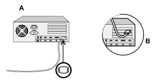
If you are using a workstation, you may need to use a 13W3 cable. Refer to *Installing a 13W3 Cable* on page 26 for instructions.
