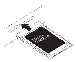
Figure 1. Smart card installation
