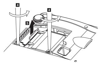
6. Pull firmly on the module handle to remove the lamp module as shown in 6.
