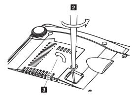
4. Remove the two screws from the lamp module as shown in 4.
