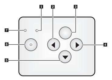
Figure 1-4. Keypad on projector
