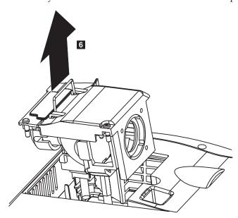
7. Reverse steps 1 through 5 to install the new lamp module.
