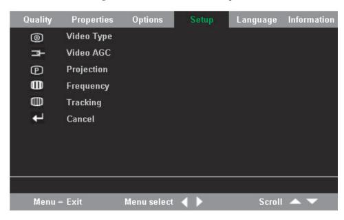
3. Press the cursor up/down button to move up and down in the Setup menu.
