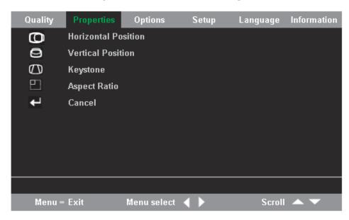
3. Press the cursor up/down button to move up and down within the Properties menu.
