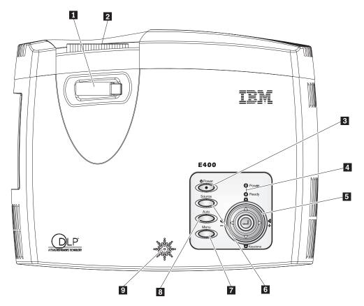
Figure 1-2. Top view of projector
