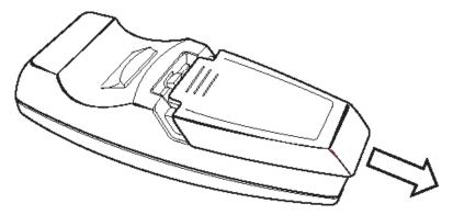
2. Insert the supplied batteries taking note of the polarity (+/-), as shown.
