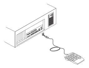
Attach the keypad cable to the USB port as shown above. For additional information on this product, visit the IBM Personal Computing Web site at: http://www.ibm.com/pc
