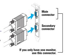
Note: With the special TV output adapter\* included with your Matrox product, you can connect a TV or video recorder to the *secondary* connector on your graphics card. For more information, see "TV output" in the online version of this guide.
