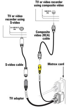
(Note: Using the Matrox composite video and S-video connectors at the same time is optional.)
