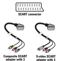
To use a SCART adapter, connect the SCART end of the adapter to your TV or video recorder, then connect the other end to your Matrox TV adapter *and* sound card.
