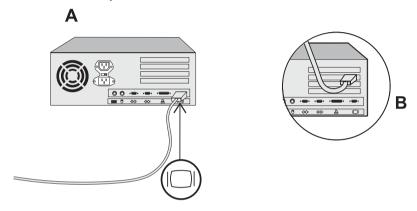
3. Connect the power cord to the power port on the back of your monitor if the power cord supplied is not attached to the monitor. Then insert the plug into a properly grounded electrical outlet.
