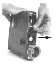
Place the projector on its side. Grasp the pull tab to pull the lamp out. Dispose of the lamp module in an environmentally proper manner.
