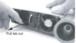
Place the projector rightside up on a flat surface. Pull the yellow tab on the lamp outward. This disengages the lamp connector.
