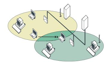
Figure 1-1. Multiple Cell Network
