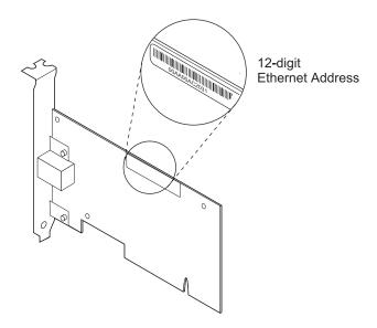
Figure 2-2. Ethernet Address Location
