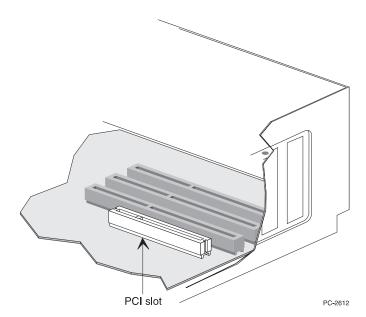
Figure 2-1. PCI Slot Illustration
