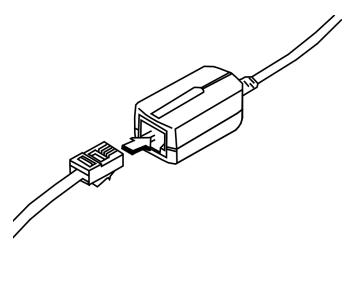
Figure 1-3. Connecting to the Network Cable to the LAN Adapter Cable
