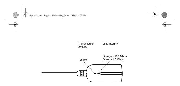
Figure 4-1. LAN Adapter Cable (100BASE-TX/10BASE-T)
