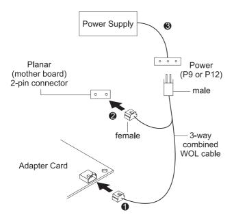
Figure 4. Connecting the 3-Way Wake On LAN Cable
