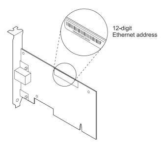
Figure 2. Ethernet Address Location
