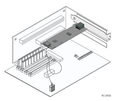
Figure 3. Connecting the 2-Way Wake On LAN Cable
