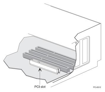
Figure 1. PCI Slot Illustration
