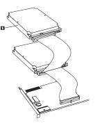
The connector on one end and the connector in the middle connect to the storage devices. The other end of the cable connects to the IDE port. The IDE port can be on the computer system board or on an adapter installed in an expansion slot. For the best signal quality when you have only one device on the IDE cable, connect the device to the connector on the end opposite the IDE port.
