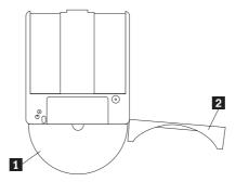
To return the disc to the Type II cartridge, align the label side of the disc **1** with the DVD-RAM cartridge label side. Insert the disc and close the cartridge lid **2**. A clicking sound will ensure the lid door is closed.
