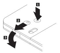
Using the tip of a ball point pen, push and break the lock pin tab 1. To remove the disc, use a ball point pen to push down on the cartridge lid lock 2 and pull the cartridge lid out to eject the disc. With the cartridge lid 3 open, the disc will eject. Do not touch the recording side of the disc when handling the bare media.
