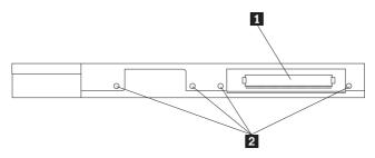
**1 Power/Data connector:** This connector provides power to the drive and data signals to the computer
