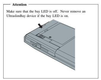
2 Slide the UltraslimBay device lock to the unlock position 1; then remove the diskette drive 2.
