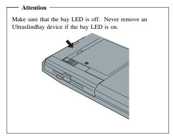
Slide the UltraslimBay device lock to the unlock position **1**; then remove the diskette drive 2.
