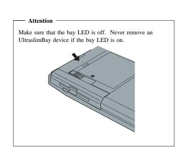
2 Slide the UltraslimBay device lock to the unlock position 1; then remove the diskette drive 2.
