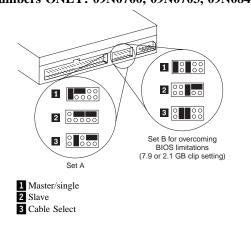
The IBM Enhanced IDE 6.4, 10.1, and 12.8 GB Hard Disk Drives offer a choice of jumper configurations, so that the drive will function properly on the widest range of computers. In some computers, the BIOS (Basic Input Output Software) will not recognize a hard disk drive reporting more than a fixed capacity, such as 2.1, 4.2, 7.9, or 8.4 GB. The following instructions will help you determine if your computer has this kind of BIOS, and what configuration settings your computer requires.
