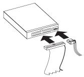
When you connect SCSI drives to the SCSI adapter, start with the SCSI connector on the cable that is farthest from the adapter. Then, with each additional device, work your way in from the far end back towards the adapter. Connecting the devices in this order ensures better signal quality. Connect the SCSI cable to the tape drive. Connect the power cable to the power connector.
