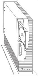
**Note:** When using your computer with the floor stand, secure CDs in the CD-ROM drive using the clips on the tray so the CD does not fall out. The above illustration shows a CD installed in the loading tray of the CD-ROM drive. The loading tray pictured has extendable clips. Your loading tray might have extendable clips or might have stationary clips.
