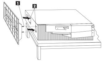
b. Push the floor stand 1 firmly into the computer, inserting the hooks fully into the slots. Slide the floor stand toward the back of the computer until it clicks into place.
