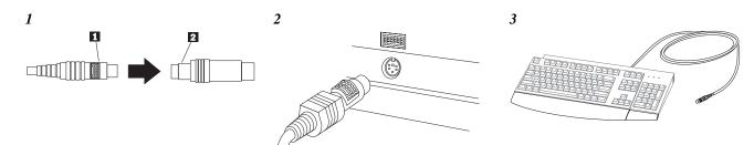
I Turn off your computer and all attached devices. If you have another keyboard attached, disconnect it. If your computer has a 5-pin keyboard port, attach the included adapter 2 to the keyboard cable 1, as shown above.
