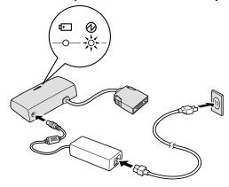
4 Place the label side of the battery pack face up, press the connector release buttons, and then connect the adapter to the battery charger.
