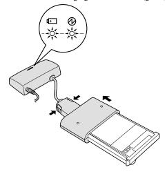
${\bf 5}$  When the charging indicator turns off, the battery pack is fully charged.
