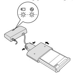
5 When the charging indicator turns off, the battery pack is fully charged.
