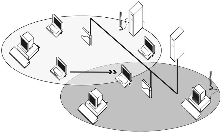
All wireless stations within this coverage area that wish to connect to the network must be configured with the same network name as the Access Points.
