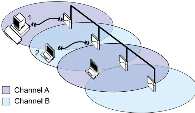
This way you can apply a maximum channel separation for neighboring Access Points that will easily satisfy the requirements recommended for optimal operation.
