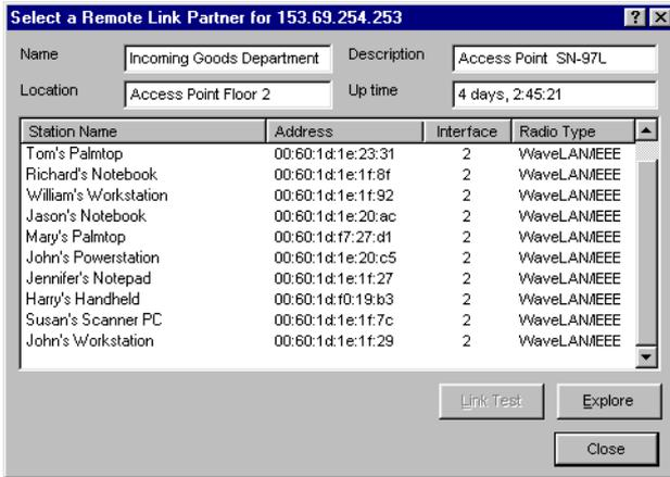
The middle section of the “Select Remote Link Partner for ...” window displays all wireless devices connected to the “initiator station”. The following fields are visible:
