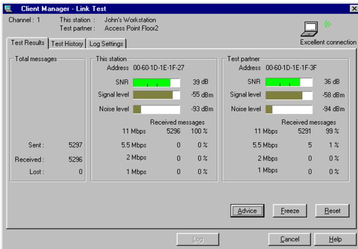
The “Link Test” window provides you with three link test options to assist you in analyzing the link test data:
