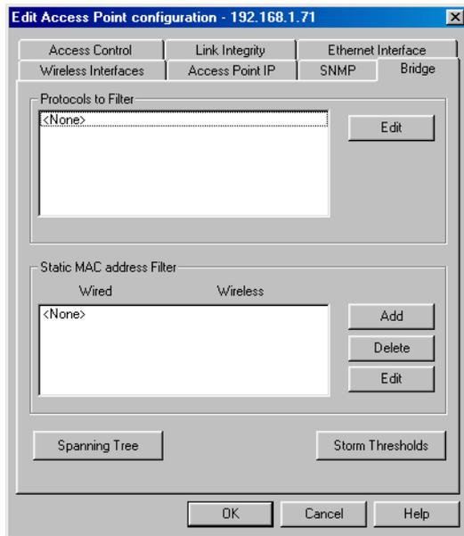
To set the Bridge parameters, connect to the Access Point and select the **Bridge** tab to display the bridge parameters as pictured in Figure 8-1.
