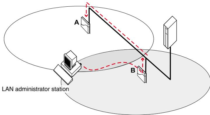
When looking at the scenario pictured in Figure 3-4 on page 3-9, the wireless network interface of the LAN administrator station should be configured to match the settings of Access Point **B**.
