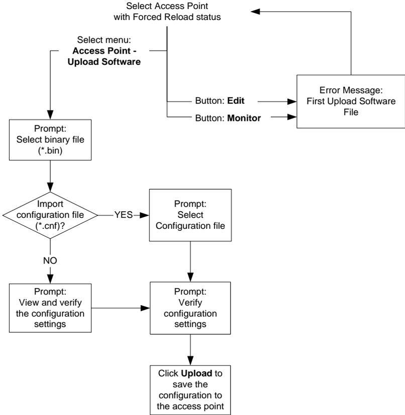
To configure the Access Point in forced reload status and to upload the configuration perform the following steps:
