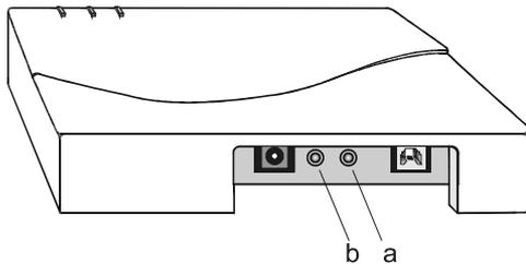
3. Use a small pointed object, such as the tip of a ball-point, to press the **Reset** button.
