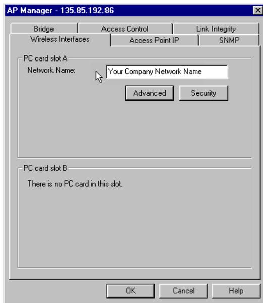
2. Enter the identification designator in the field **Network Name** for the service type that this interface should use:
