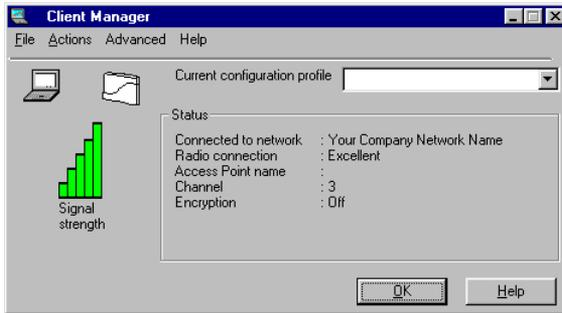
The main Client Manager window will display the key information required to validate the current network connection of your High Rate Wireless LAN station:
