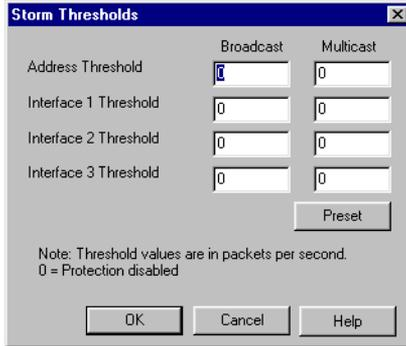
The factory-set configuration for storm threshold protection is disabled (all values are set to zero).
