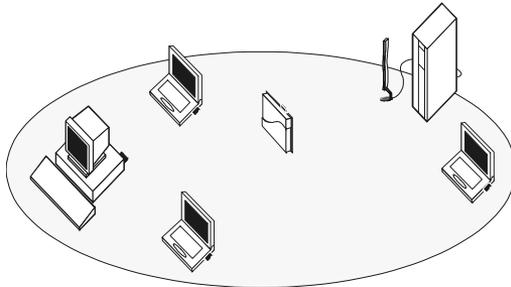
The wireless infrastructure is identified by a unique network name. All equipped devices that wish to connect to this network, must be configured with an identical network name.
