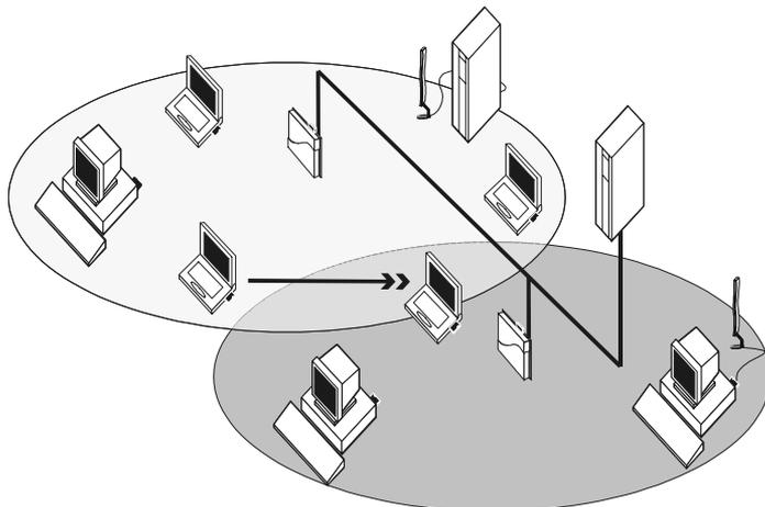
To connect a wireless station to the High Rate Wireless LAN network, each station must be configured with the same Network Name as the Access Point.
