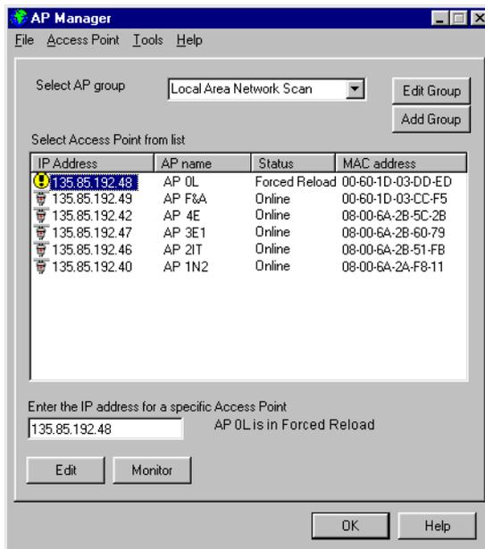
2. Select **Upload Software** from the Access Point menu to start the configuration and upload procedure.
