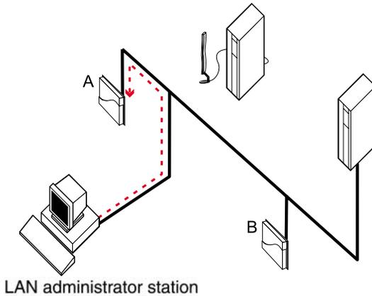
Looking at Figure 3-2, the LAN administrator station has access to both Access Points **A** and **B** via the wired backbone.
