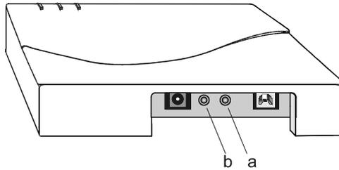
3. Use a small pointed object, such as the tip of a ball-point, to press the **Reset** button. The Access Point will restart and run the start-up diagnostics, characterized by a LED sequence where the LEDs change color in the range Red, Amber, Green.
