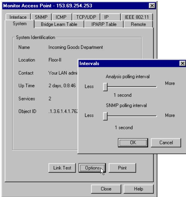
In the Intervals window two different time interval parameters can be set to change to monitor interval settings:
