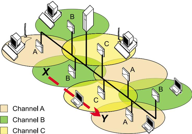
For example, looking at Figure 6-5, to set up a three channel system you could configure the Access Points as follows:
