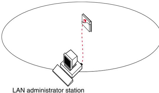
Using a wireless LAN administrator station allows you to configure Access Points:
