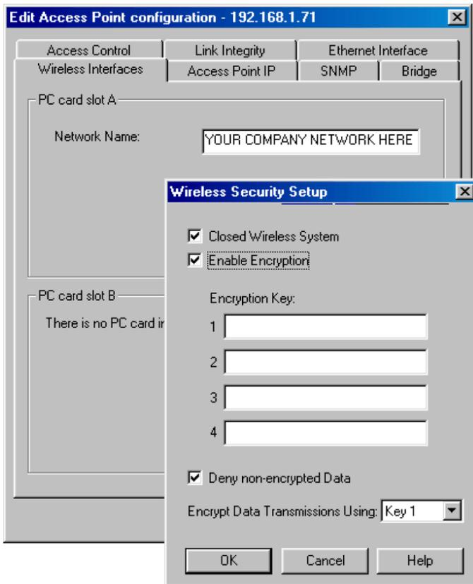
Wired Equivalent Privacy (WEP) data encryption enables you to encrypt all data that will be transmitted via the wireless LAN medium.
