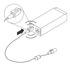
Note: To remove the in-flight power connector from the adapter, grasp the connector sleeve and slide it backwards to unlock the connector. Continue to pull the connector sleeve to remove the connector. To prevent damage, do not pull on the cord to remove the connector.
