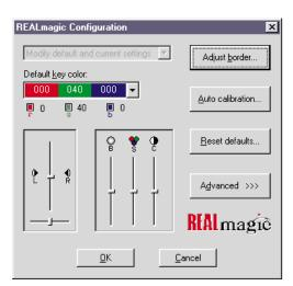
In the dialog box, click **Auto calibration...** The display will flicker for approximately thirty seconds. If the auto calibration does not adjust the border correctly, go on to the next step.
