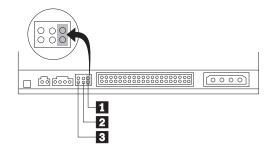
The illustration above shows the master 1 setting and the slave 2 setting. The other jumper setting is the cable-select 3 setting, which is not used on IBM computers. Configure the DVD-ROM drive by placing a jumper in the master setting.
