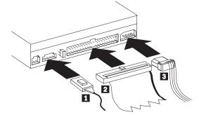
1. Connect the larger end of the included internal audio cable 1 to the audio output connector on the DVD-ROM drive. Here is an illustration of the internal audio cable.
