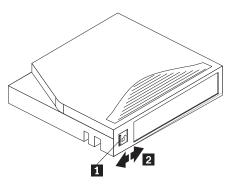
The front of the cartridge has an orange write-protect switch **1** to prevent accidental erasure. Slide the switch to the right to write-protect **2** or to the left to enable writing.
