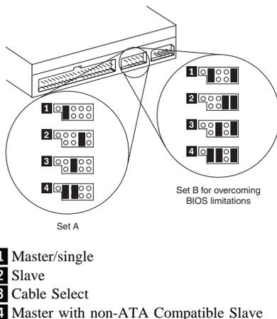
Figure 4. Maxtor manufactured drives
