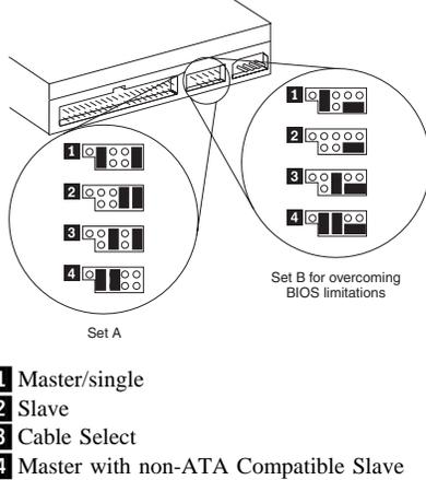
Figure 2. Quantum manufactured drives
