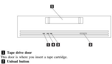
This button, when pressed, unloads a tape cartridge from the drive.
