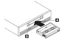
The tape drive loads the tape in approximately 20 seconds. When the tape-drive presence (green) indicator lights steadily, the tape drive is ready for read and write operations.
