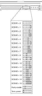
If you choose the default SCSI address of 6, go to Step 4. If you need to change the SCSI address, refer to the SCSI ID settings shown in the illustration. Remove and reposition the jumpers that come with your tape drive to set the ID. If necessary, use a pair of needle-nose pliers to remove the jumpers.
