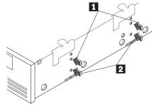
2. Align the top set **1** or the bottom set **2** of screw holes on the drive mounting rails with the drive-bay screw holes.
