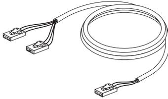
1. Connect the single-connector end of the included internal audio cable **1** to the audio-out connector on the DVD-ROM drive.
