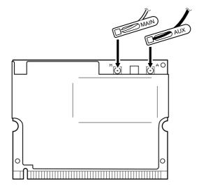
**Note:** Plug the gray antenna cable with the tab marked "**MAIN**" into jack M, and the black antenna cable with the tab marked "**AUX**" into jack A.
