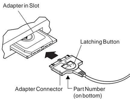
Step 5. To lock the adapter cable securely, move the latching button in toward the adapter. In some cases, you may want to leave the adapter cable latch retracted. If the adapter cable is pulled, it will disconnect from the adapter, possibly saving your computer from being pulled off a table.
