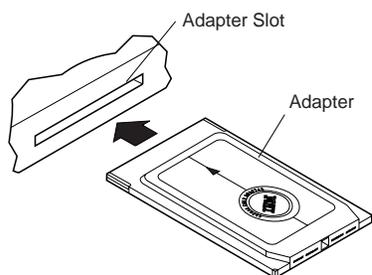
The adapter is keyed to go in one way only. If you feel resistance before the adapter is fully inserted, remove the adapter, turn it over, and reinsert it.
