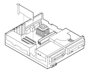
3. Install the adapter and insert the retaining screw.
