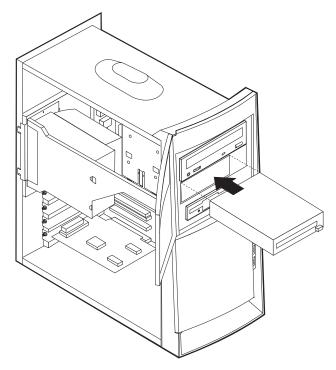
6. Each integrated drive electronics (IDE) drive requires two cables; a four-wire power cable that connects to the power supply and a signal cable that connects to the system board. You might also have an audio cable to connect.
