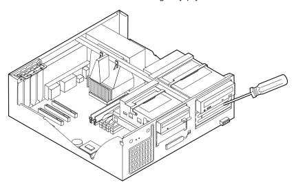
5. Pivot the drive bay latch handle toward the front of the computer and pivot the drive bay cage toward the front of the computer until the drive cage latch catches to the chassis.
