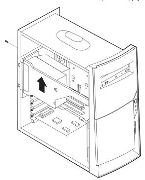
3. Rotate the power supply outward as shown.
