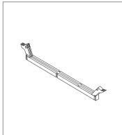
4. Make sure the notches in the DIMM align with the tabs on the connector. Push or insert the DIMM straight down into the connector until the retaining clips close.
