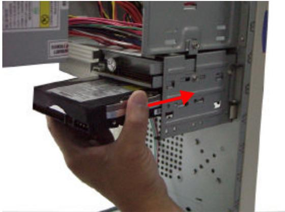
**3.**For the hard disk drive, follow the same manner for installing the floppy disk drive.
