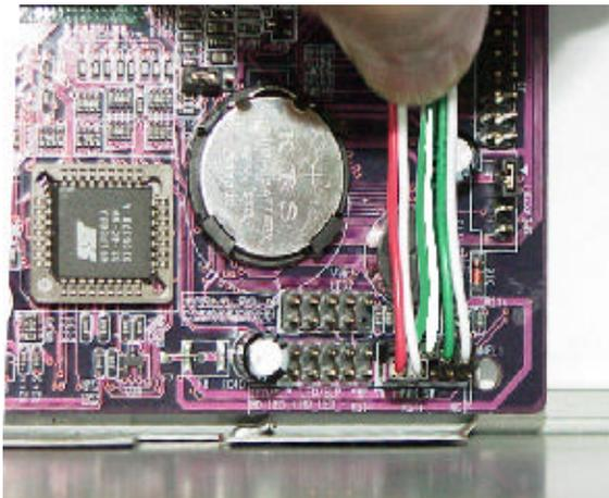
The Power SW and HDD LED should look like this after they are connected.
