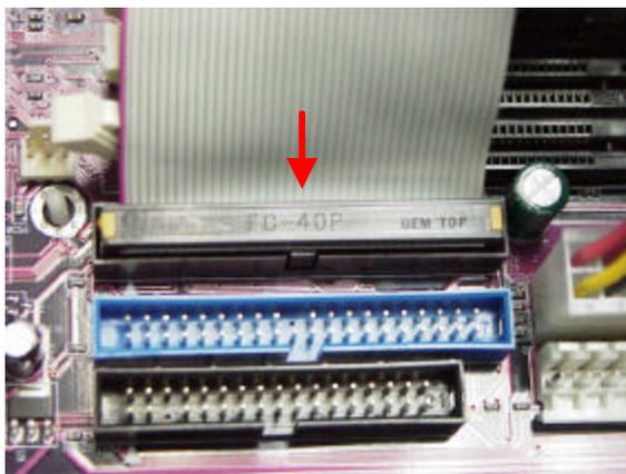
**9.**Plug the CD-ROM cable into the Primary IDE channel on the mainboard. The edge of the cable that is red determines its orientation. Push the CD-ROM cable squarely onto the Primary pins.
