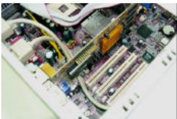
**18.** Install the AGP card back to the expansion slot. Situate the cables below the AGP card.
