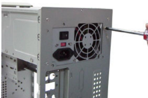
**2.** Using the screwdriver, gently tighten the three screws. This completes the installation for the power supply fan.
