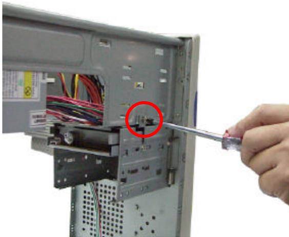
**8.** Secure the chassis and the storage bay with screws. Do not over tighten the screws. Gentle pressure is enough.
