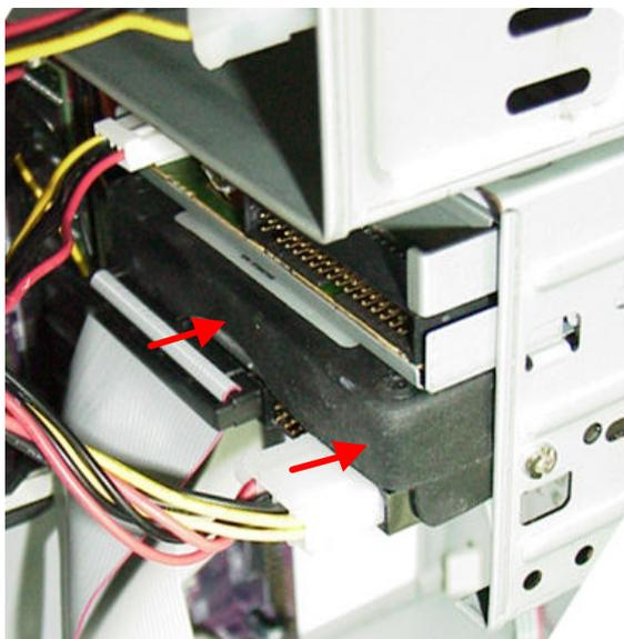
**12.** Following the same procedure mentioned in step 10. Connect the other end of the cable to the hard disk drive.
