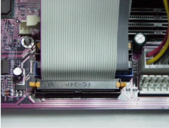
**13.** Lastly, connect the cables of the floppy drive as you did with the CD-ROM and hard disk drive. The edge of the cable that is yellow should situate firmly on the plastic shroud.
