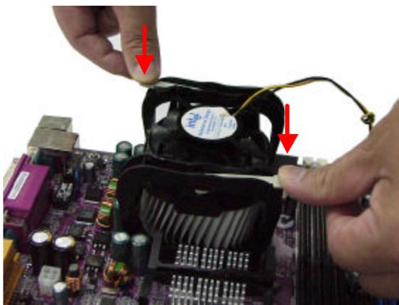
**7.** Lock both levers on top of the cooling fan to their opposite sides to secure the cooling fan on top of the heatsink.
