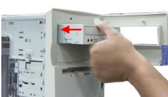
**5.** Slide the CD-ROM drive into the bay and align the drive's faceplate with the front of the case.
