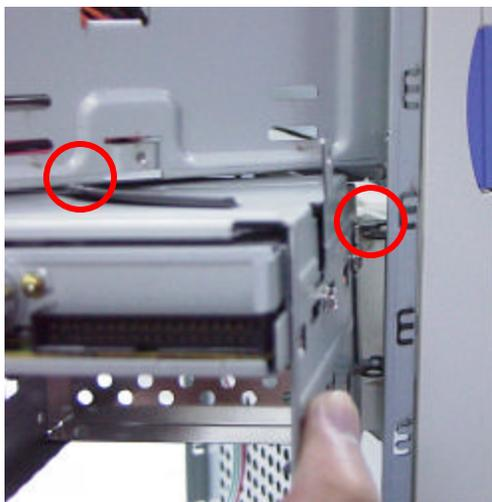
**6.** Push back the storage bay to its original position. There are two things that need to be aware of: One is to make sure that the screw holes of the mounting box are aligned with that of the drive and the brackets are smoothly attached to the hook.
