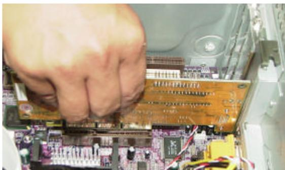
**2.** Following the figure, push the edge connector of the AGP card into the expansion slot.
