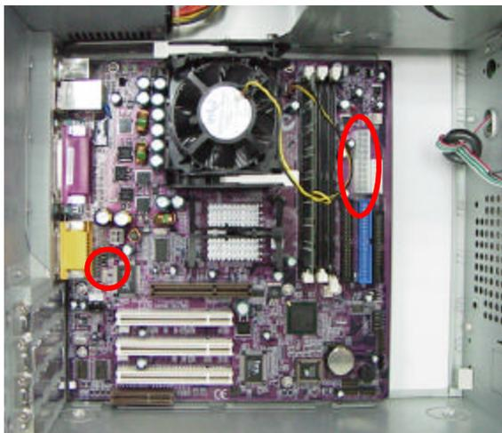
**3.** Locate the mainboard power connector. See figure for reference.
