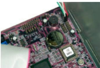
**14.** Locate the USB2 header on the system board.
