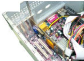
**3.** The figure shows the system board inside the case.
