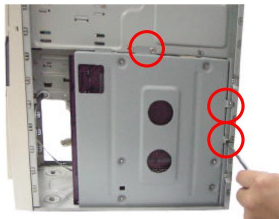
**13.**Secure the mainboard into the mounting brackets with screws. Do not overtighten the screws. Gentle pressure is enough.
