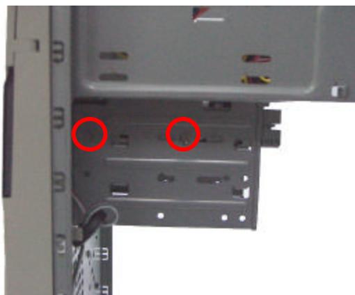
You can easily see where the screw holes in the drive line up.
