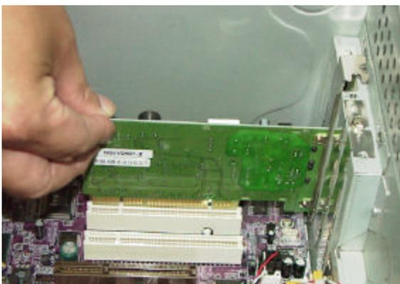
**5.**Next, install the Modem card as the same way with the AGP card. Insert the Modem card to the first 32-bit PCI slot. Refer to the figure for reference.
