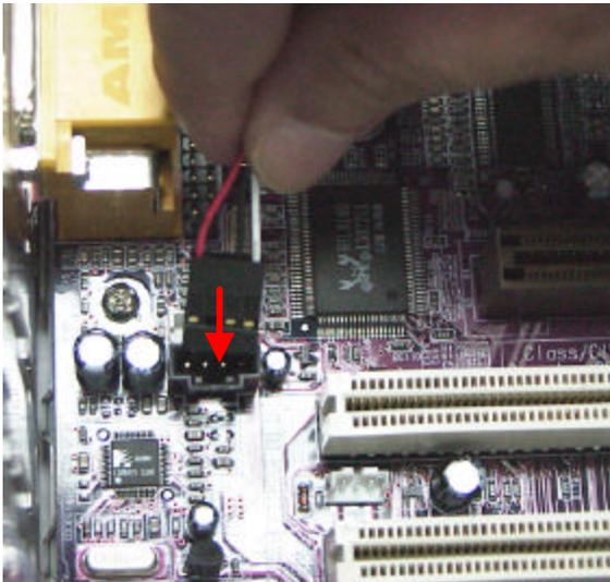
**16.** Attach the other end of the cable to the controller on the mainboard. See figure for reference.
