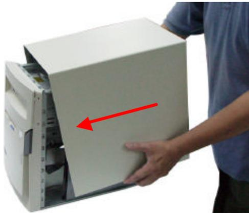
**1.**When all necessary peripherals and drivers are installed in the case and that there are no loose wires that may get in the way of the CPU fan and other components. Place back the top cover to the case.
