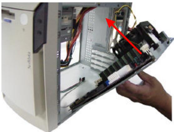
**12.**Place the mainboard over the mounting brackets. Then slide the mainboard into place as shown in the next figure.
