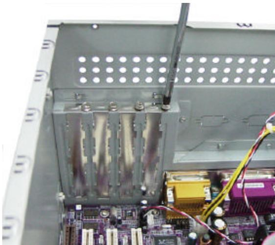
**1.** The most commonly used expansion card is the AGP and modem card. Let's start by installing the AGP card first. Remove the dust cover from the slot in the system case that corresponds to the expansion slot that you are going to use.
