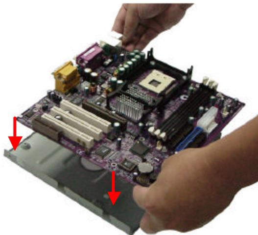
**2.** Position the mainboard in the plate so you can see the alignment of the mounting holes in the mainboard with the standoff holes. There are at least 4 screws that need to be secured.
