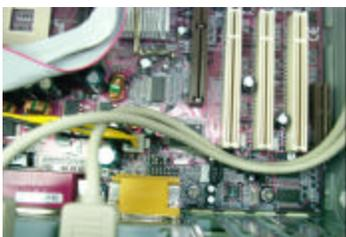
**17.** To reduce unnecessary tangles, place the cables beside the slots as shown in the figure.
