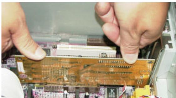
**3.** Using both hands, gently press down the AGP card firmly to ensure that the edge connector is correctly rested in the slot.
