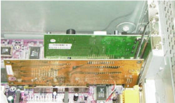
You have finished installing the Modem and AGP cards. Make sure that the add-on cards are installed properly on the mainboard See figure for reference.
