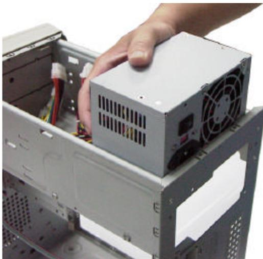
**1.** The power supply should be installed in the back of the chassis. This is to draw the air out of the inside of the case. Check the position of the power supply fan as shown in the figure.
