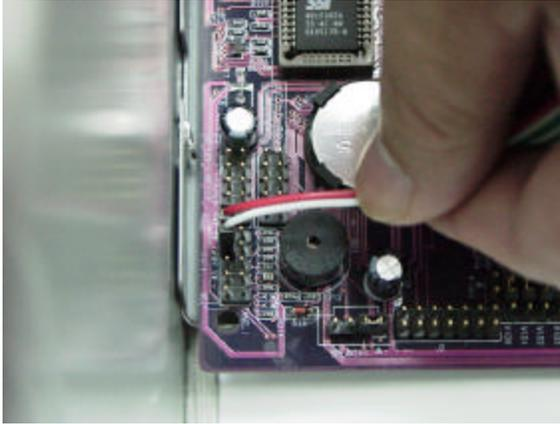
**4.** Next, Connect the HDD LED into the connector of the mainboard. The HDD LED indicator has two pins with one of them marked positive. One of the wires from the HDD LED is usually red and goes on the positive pin.
