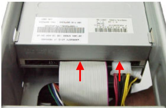
**10.** Connect the other end of the cable to the CD-ROM drive. Note the orientation of the cable before trying to connect it.
