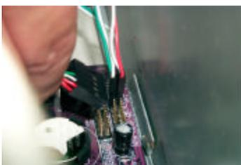
**15.** Connect the USB connector into the USB2 header of the system board. Note that the connector is keyed (Pin 9) so that it can only be installed correctly on the header.
