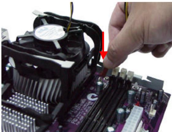
**8.** Connect the CPU cooling fan power cable to the CPU fan connector.
