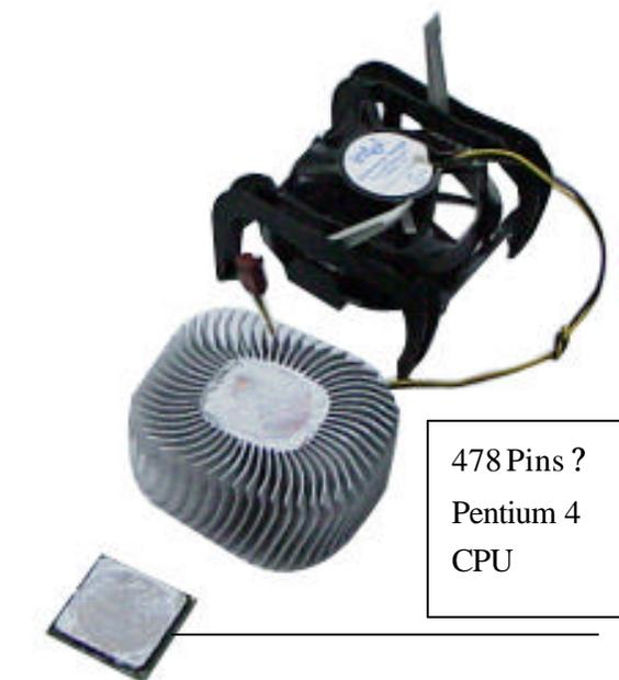
**3.**Prepare the CPU, heatsink and the CPU cooling fan.
