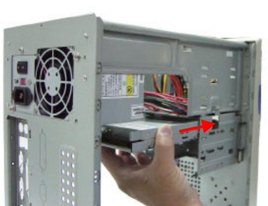
**1.** There are two different size "bays" into which each of the various drives will fit. Take a close look at the drive and determine which is the "bay" for the floppy drive. Install the floppy drive into the upper side of the storage bay. See figure for reference.
