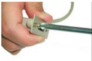
**6.** Then, loosen the screw on the other side.
