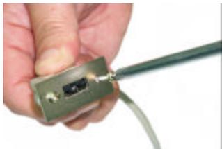
**5.** Remove one screw from the USB bracket using a screwdriver.
