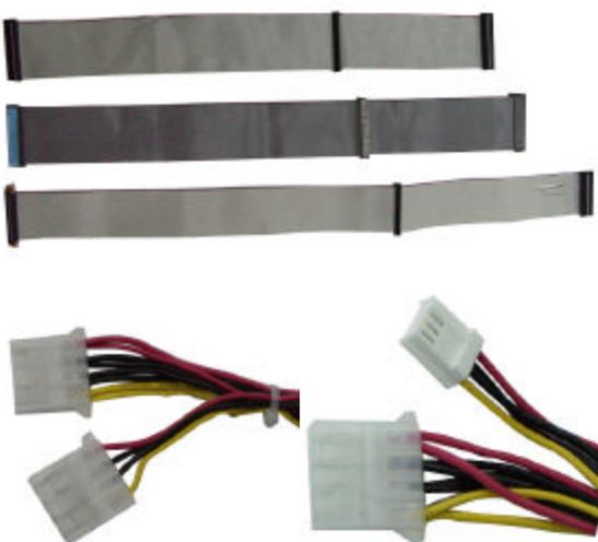
**8.**Next, you should get familiar with the cables that are used with the various drives. The first cable is use for the floppy drives, the second cable is for the hard disk drive and the third long cable is use for the CD-ROM drive. For the power cables, the cable has peripheral and floppy drive power connector and is designed to connect from the power supply to the drives.
