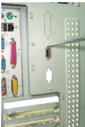
**8.** Attached the bracket and USB cable to the USB port. Make sure that the direction is installed correctly.
