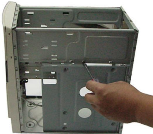
**4.** For installing the mainboard, locate the three screws which secure the plate and remove it.
