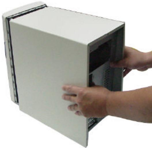
**3.** Using both hands, gently pull back the top cover as shown in the figure. Slide the cover up off the frame of the case.
