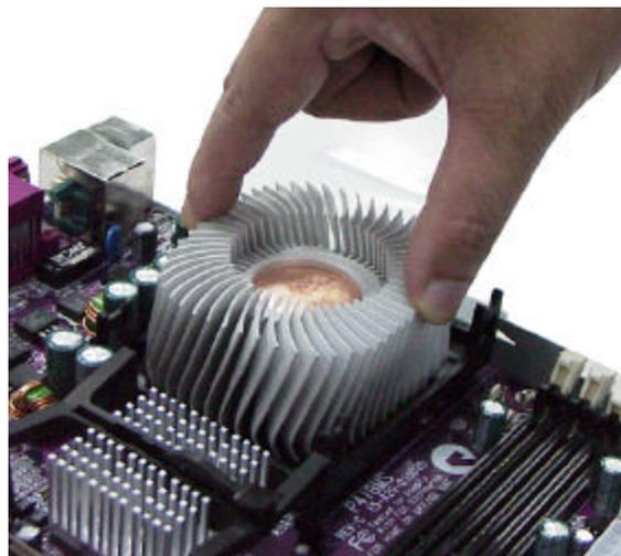
**5.**Place the heatsink at the top of the CPU. See figure for reference.
