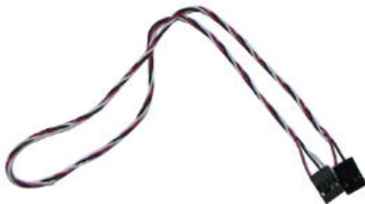
**15.** Use the audio cable provided with the CD-ROM drive to connect the audio connector on the rear edge of the CD-ROM drive to one of the audio-in connectors on the mainboard. The audio sound does not come from the mainboard itself.
