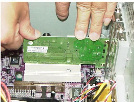
**6.**Gently use both hands to press down the Modem card onto the PCI slot.
