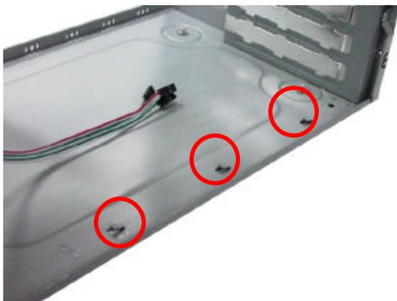
**11.**To install the mainboard inside the case. Locate the three mounting brackets on the case as shown in the figure.
