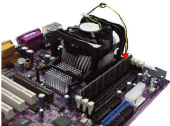
**10.**After installing, the Memory Module should look like this.
