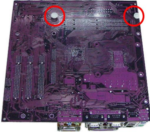
**1.** The plastic spacers provide extreme support in areas of high mechanical stress on your mainboard. Insert the plastic spacers in the 2 mounting holes as shown in the figure through the back of your mainboard. The plastic spacers are provided with the case.
