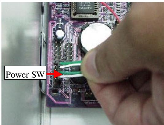
**2.** Connect the Power SW (usually with green wires) into the connector of the mainboard.
