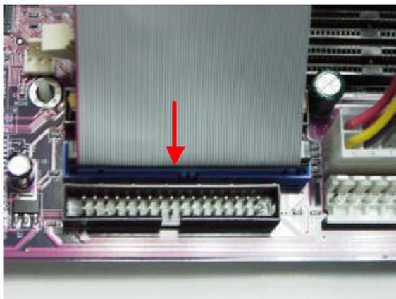
**11.** Next, plug the hard disk cable into the Secondary IDE channel on the mainboard. The edge of the cable that is red determines its orientation. Push the hard disk cable squarely onto the Secondary pins.
