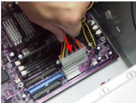
**4.** The power connector should fit perfectly in the slot on the mainboard. Note the orientation of the cables before trying to connect them. Each function of the cable is already defined.
