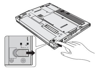
4. Slide and hold the battery latch 1; then remove the battery 2.
