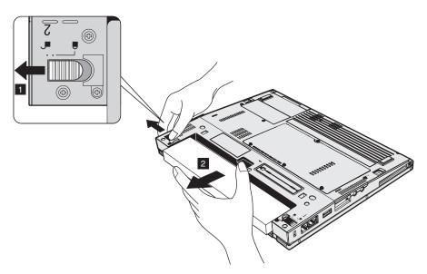
5. Align the front of a fully charged spare battery with the front side of the battery space in the computer; then gently push the battery into the space.
