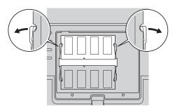
**9.** Replace the memory slot cover by aligning the back side of the cover first and then tightening the screws.
